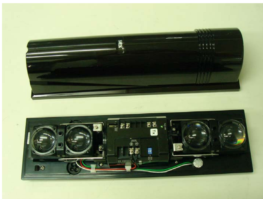
Inside view of EUT (Transmitter)
