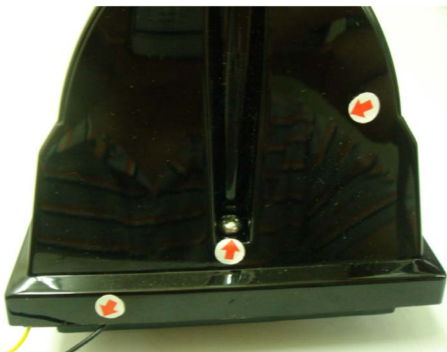
View of ESD test point
